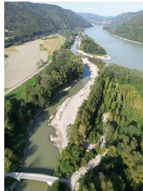
Land removal along the right riverbank at Danube side arm Schallemmersdorf and Grimsing, Lower Austria, September 2024 © Land NÖ Abt. WA3 Nesweda
